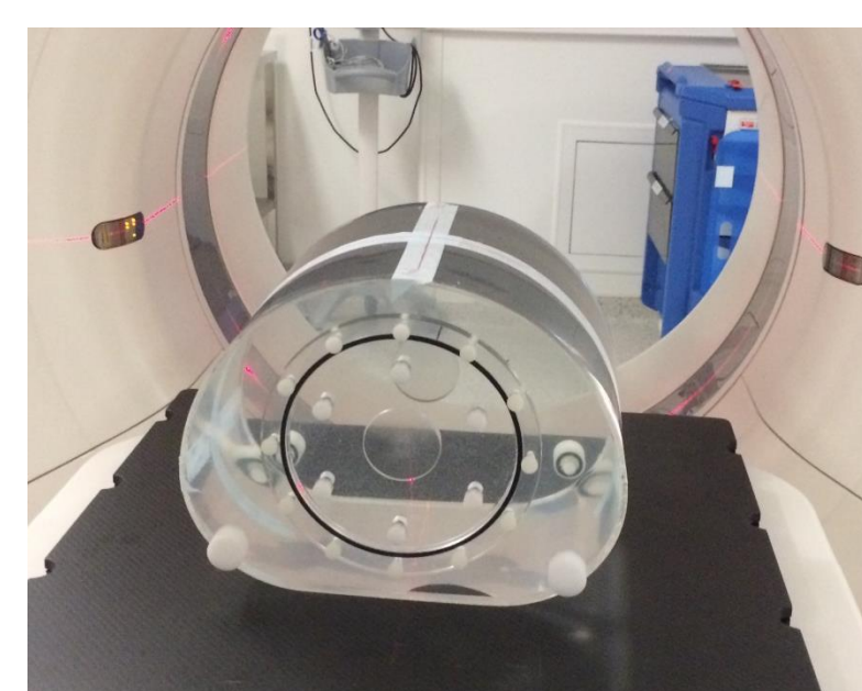
Figure 1: Phantom without multiple fillable spheres and cylindric inserts and fill with water
